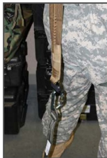
QRET Connection to Modified PRT
