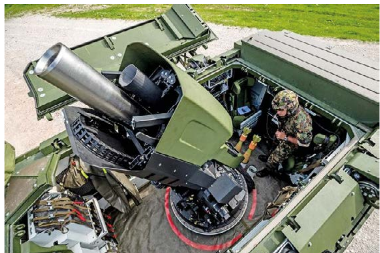
Mortero COBRA con carga semiautomática. Foto Swiss Ministry of Defense, officially called the Federal Department of Defense, Civil Protection and Sport
