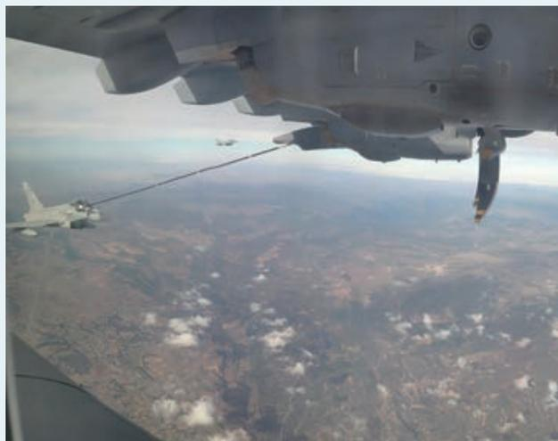
*EDA Research into Automatic Air-to-Air Refueling for Hose and Drogue System | EDA*
