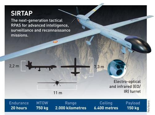
Designed to fly in the most adverse weather and operating conditions, both on land and at sea, the UAV will be capable of conducting day and night operations, take-off from short, unpaved runways, and will be certified to operate in segregated airspace.
